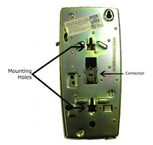
Some wall jacks may not be compatible with the sliding jack version of the 2554. Cortelco recommends the following jacks:
