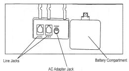
3. Plug power transformer into a non-switched electric outlet, then plug the connector into the base.
