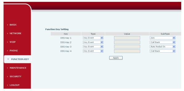
Memory Key – Select Type as Memory Key and enter the number to be dialed in the Value box. When the key is pressed, the phone will dial the programmed number. Key Event – Select Type as Key Event and then select the SubType from the following options:
