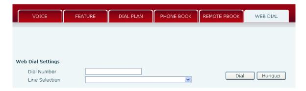
This feature allows a call to be initiated by a computer. To place a call, enter the number in the Dial Number box, select the line in the Line Selection box and press the Dial button. To end the call, press the Hangup button.
